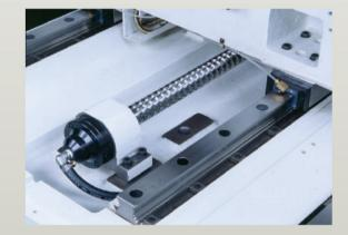
■ The 3-axis transmission guide rod system employs hollow cooling design to minimize heat and thermal expansion of ball screw in high-speed operations with cooling oils to balance high speed and high precision at the same time.
