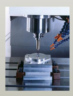
■ The standard test blocks after machining shall subject to measurement by 3D CMM (Coordinate Measuring Machine) to ensure compliance of accuracy with standard.
