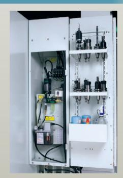
■ Centralized air compressing system and lubricating system is easy for repair and maintenance.
