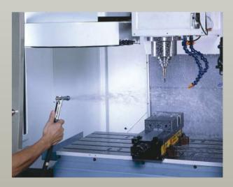
The Coolant gun for machine cleaning can remove the residual chips attached to the machine, keep the cleanness of the machine and facilitate the maintenance works.
