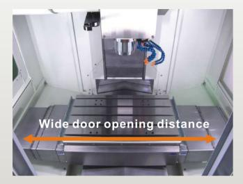
Extra-wide door, easy for loading/unloading the parts or jigs to/from the machine.
